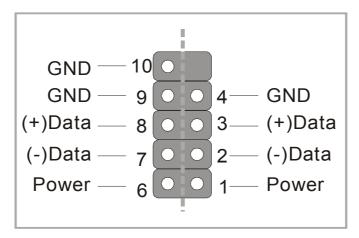
USB1, USB2, USB20\_1 and USB20\_2 support USB2.0 devices. USB20\_1 and USB20\_2 support USB2.0 devices.
